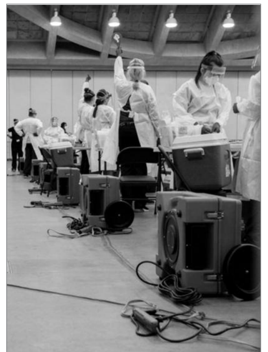
PHOTO COURTESY MARYLAND DEPARTMENT OF HEALTH Each testing station at the site has a dedicated industrial-grade HEPA filter.
